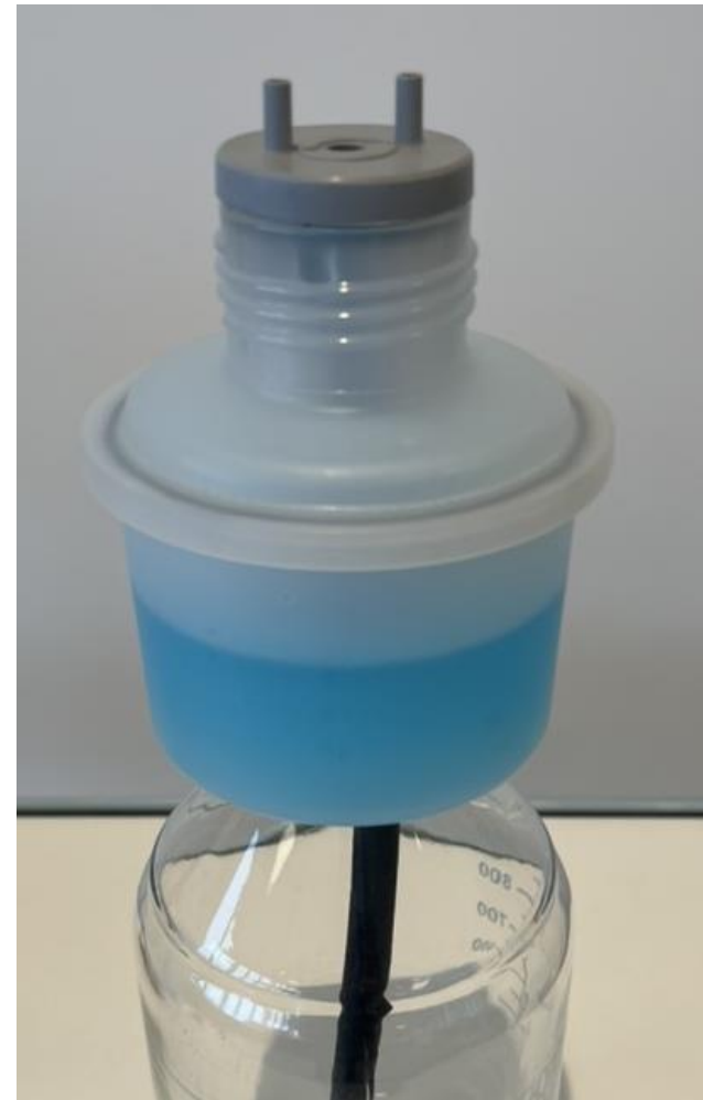
Attach the stirrer on top of the GAA
