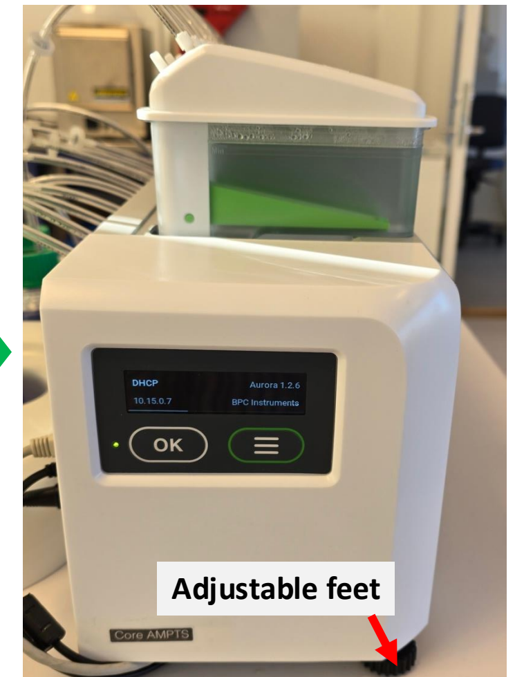
Make sure that each FCU is level on the core unit and seated correctly.
