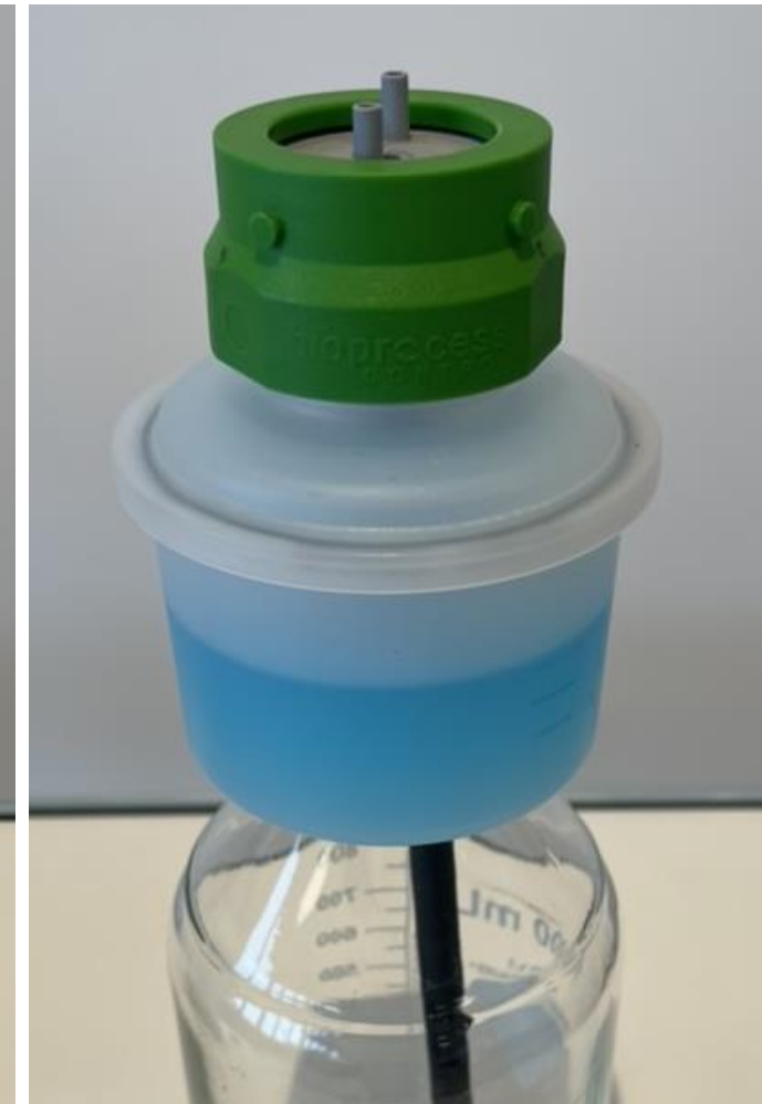
Add the bottle nut to hold the stirrer in place
