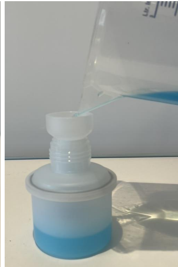
Carefully add the alkaline solution previously mixed with pH indicator until the 80 mL marked level on the GAA.
