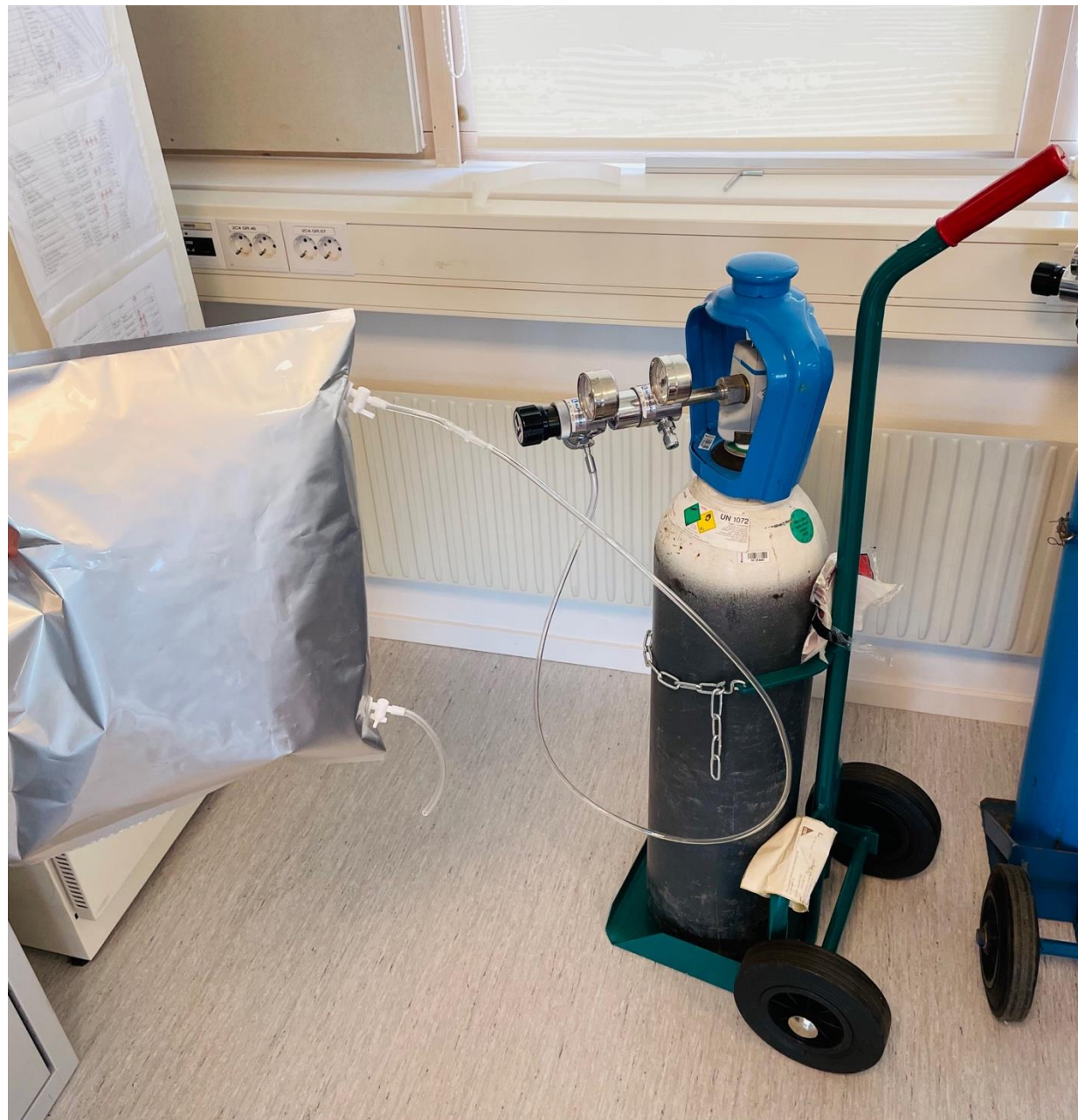
Fill up the gas bag using an oxygen cylinder equipped with a pressure regulator
