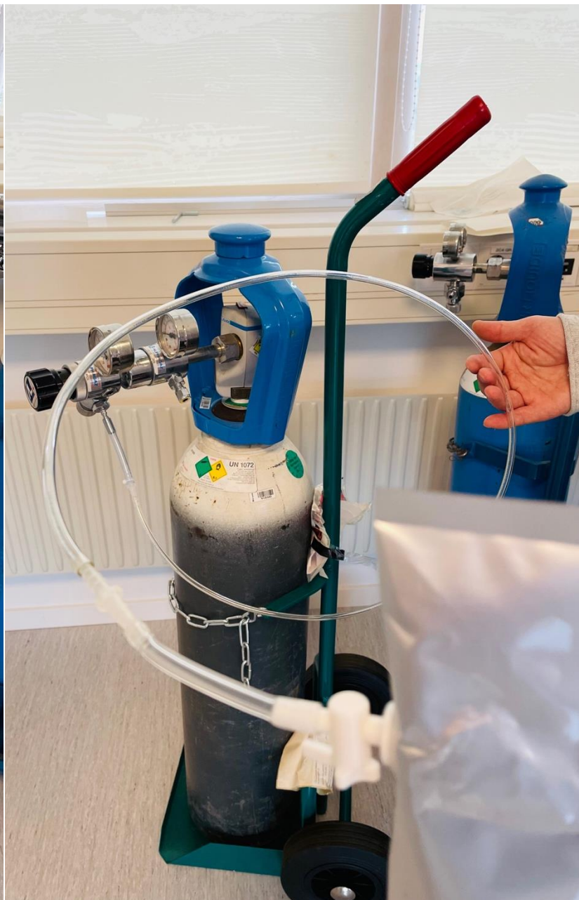
Avoid overinflating the bags as this can impact the data registration
