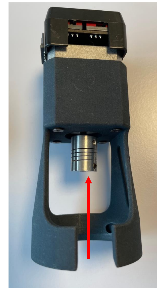
Connect the axis coupling to the motor axis
