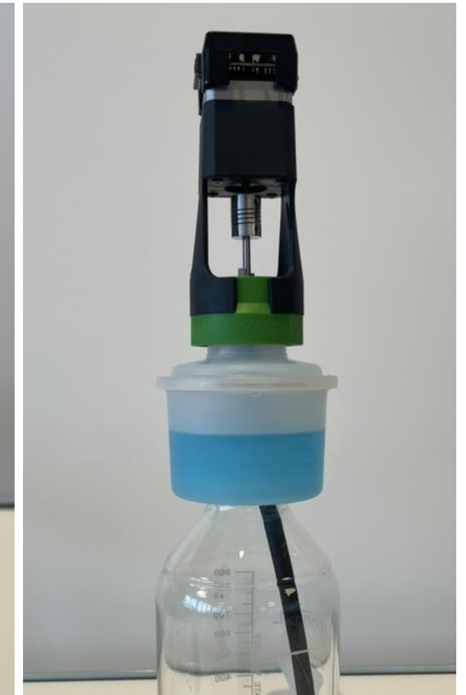
Attach the motor by placing it on the top, with the metal rod going into the bioreactor and fitting into the stirrer.
