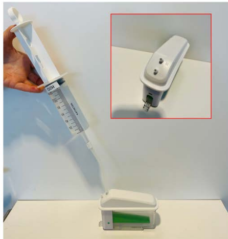
Each FCU has an inlet and outlet for the gas. Use the syringe to introduce water through the inlet of the FCU
