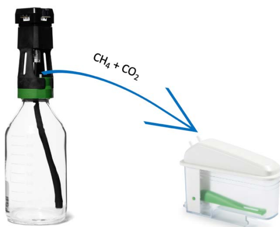
Figure 6. Setup for total gas (e.g., biogas) measurements.
