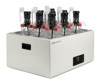
The BRS III is a laboratory-scale instrument designed to replicate continuously fed anaerobic fermentation processes. Its user-friendliness, fully automatic operation, and robust reliability make it effortless to use. Featuring 9 parallel channels, it enables the simultaneous evaluation of multiple process operational conditions.
