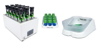
AMPTS® II lets you determine the optimal retention time and mix of substrates for co-digestion, screen proper pre-treatment methods and evaluate the need for additives.
