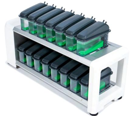
Gas volume & flow meter array and DAQ unit
