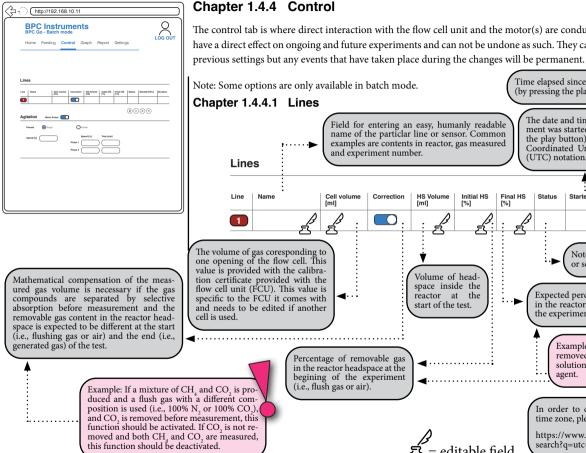
The control tab is where direct interaction with the flow cell unit and the motor(s) are conducted. All changes here will have a direct effect on ongoing and future experiments and can not be undone as such. They can be changed back to their
